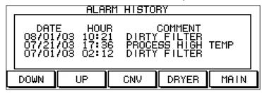
This screen allows the operator to review the number and type of issues that the Dryer has encountered during its operation. The "Alarm History" screen is NOT reset-able.
